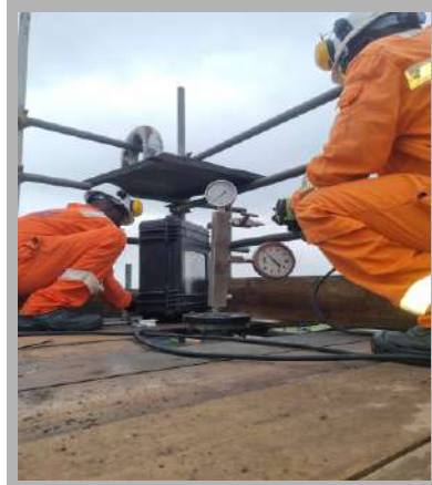
Hydrotesting a 30,000 litre capacity Diesel tank ABB GT1- SEPNU Power plant
