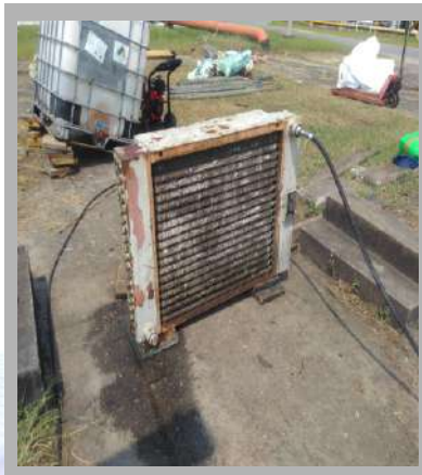
Hydrotesting an oil cooler SEPNU
