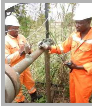
UT Measurement on a wellhead flow line
